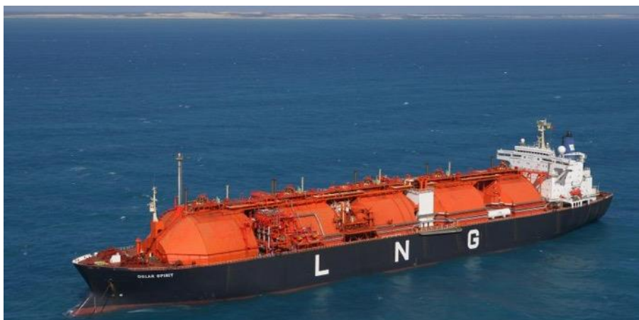
Figure 2-13 LNG Carrier with Moss Spherical Tank System
