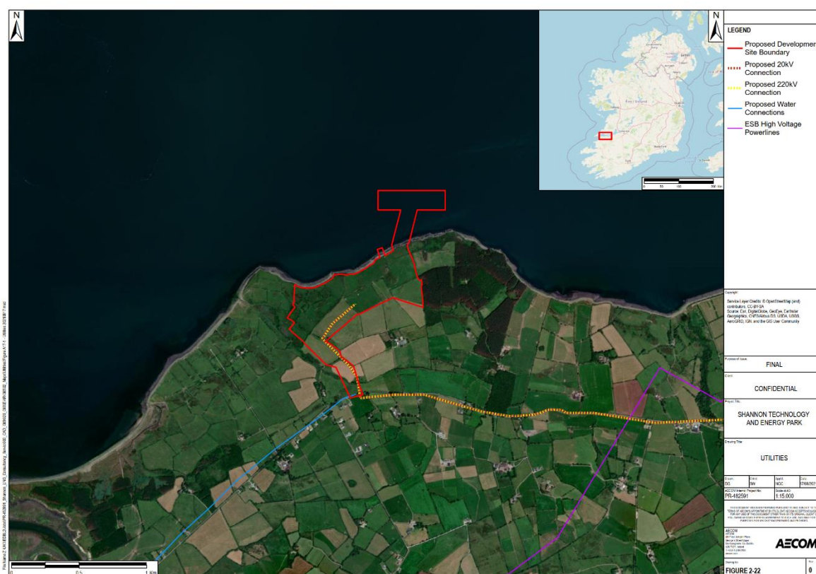
Figure 2-22 Proposed Electrical and Water Connections
